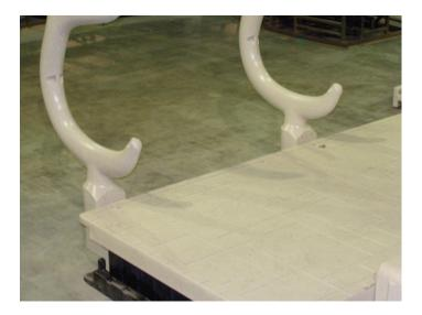
3. Store the kayaks on the Kayak rack upside down and secure with a stretch cord using the molded in eyelets in the arms.
