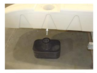
Line up the top peg with the post hole and push into place.
