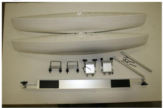
2. Assemble all parts as shown in the photos below and determine the proper location on your kayak or canoe. The stabilizer may be attached either on the front or the back half of the kayak. Determine the location based upon length of the craft and the flat area to mount the kit on. Make sure that the location keeps the floats out of the way while paddling.
