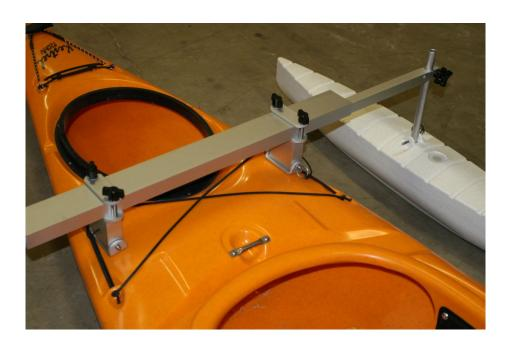
6. Attach support bar to the canoe using the angle brackets and the long u-bolts. The long side of the angle should be towards the canoe interior. It may be possible to use these same brackets to attach the stabilizer to some kayaks.
