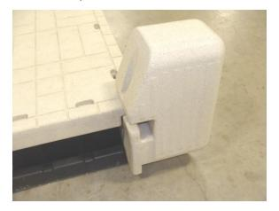
**2.** Align the bolt hole in the bumper with one of the slots in the dock at the desired location. The slots are approximately 20" apart. Secure with the  $3/8 \times 5$ " bolt and washer.
