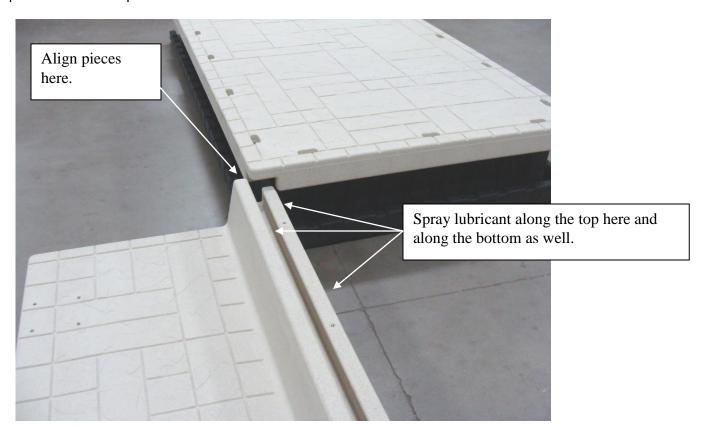
2. Slide lowered section into the dock channel. Slide it to the desired position and also be sure one of the threaded inserts aligns with the slot in the dock deck.
