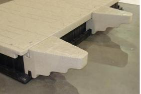
2. Position the dock bench on the attachment arms so the bolt hole in the leg lines up with the threaded insert in the attachment. Adjust the bench attachment position as necessary so they align. Secure the back legs of the bench to the attachment arms with the  $3/8 \times 13$  bolts and washers.
