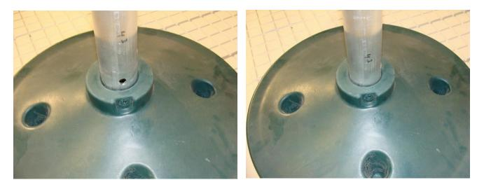
2. Insert the umbrella sleeve into the molded hole in the table top. (See Page 3. if you do not have this molded hole in the table top.) Be sure to align the holes in the sleeve with the bolt hole in the bottom of the table top. This is the same bolt hole as shown in step 1. Do not insert the bolt yet.
