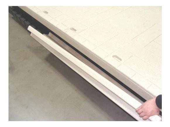
2. Bend filler piece outward in the middle so the top edge can slip into the top channel on the dock section.
