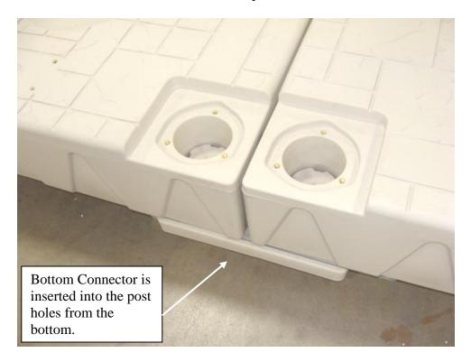
3. Insert the top connector into the post hole openings. Secure the connector pieces together using the  $3/8 \times 1 \frac{1}{2}$  bolts and 3/8 fender washers. Repeat procedure at the rear of the port.
