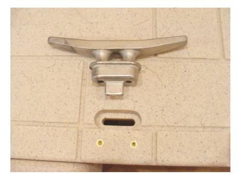
2. Insert cleat into the opening and align the bottom plate with holes in the cleat.
