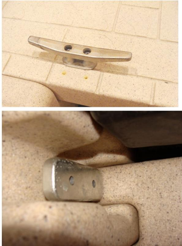
Bottom side of deck with the bottom plate in proper position.
