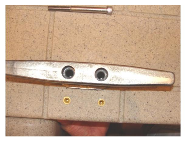
3. Insert the long bolts along with the lock washers into the holes in the cleat. Thread the bolts into the bottom plate and tighten securely.
